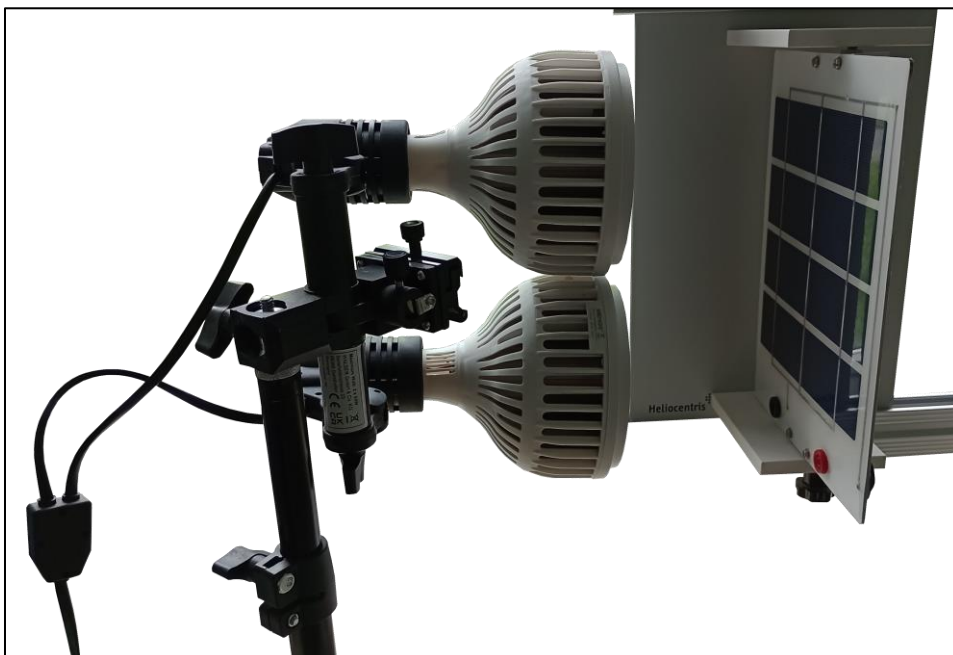
Lamp system with Heliocentris Dr FuelCell® solar panel
