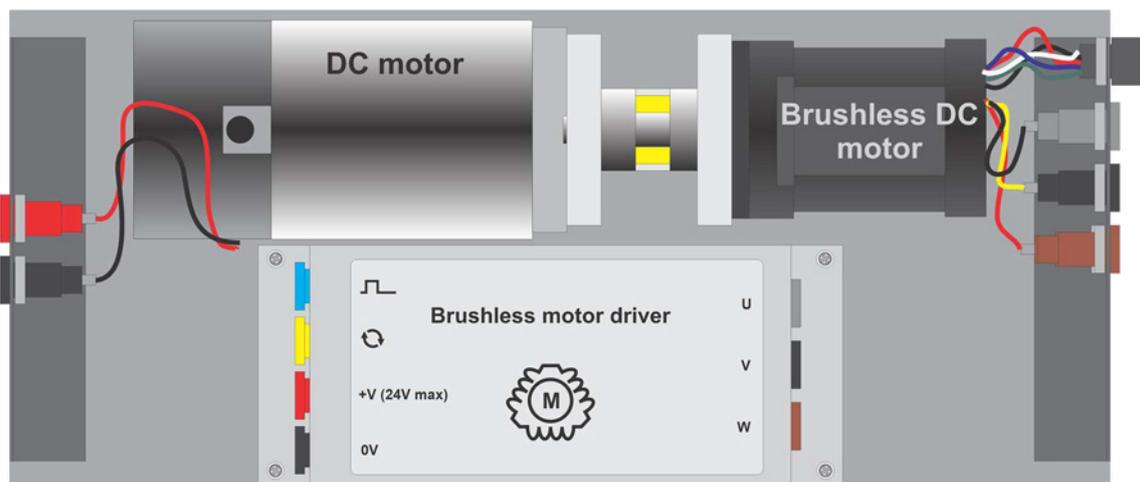
The HP2001 DC motor/brushless motor pair consists of two parts: the motors themselves, coupled together, and a brushless DC motor driver.
