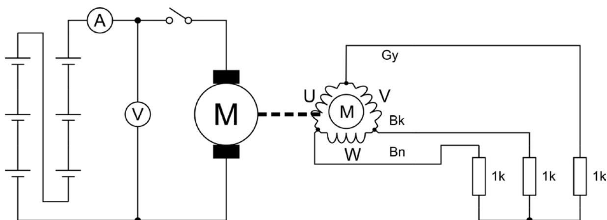
You built the circuit shown in the diagram above. In reality, it is two separate circuits. Each has its own earth or ground. They are not connected and can be at different voltages.
