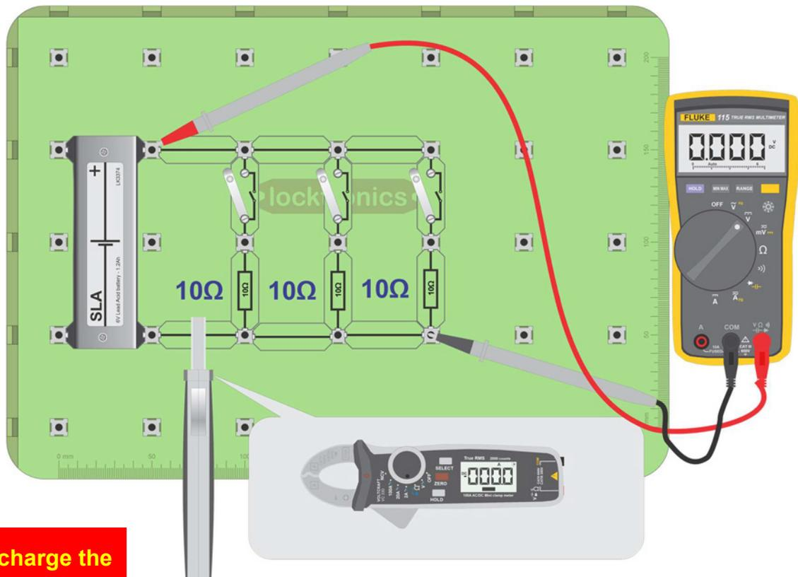
**Do not discharge the batteries below 3.2V**
