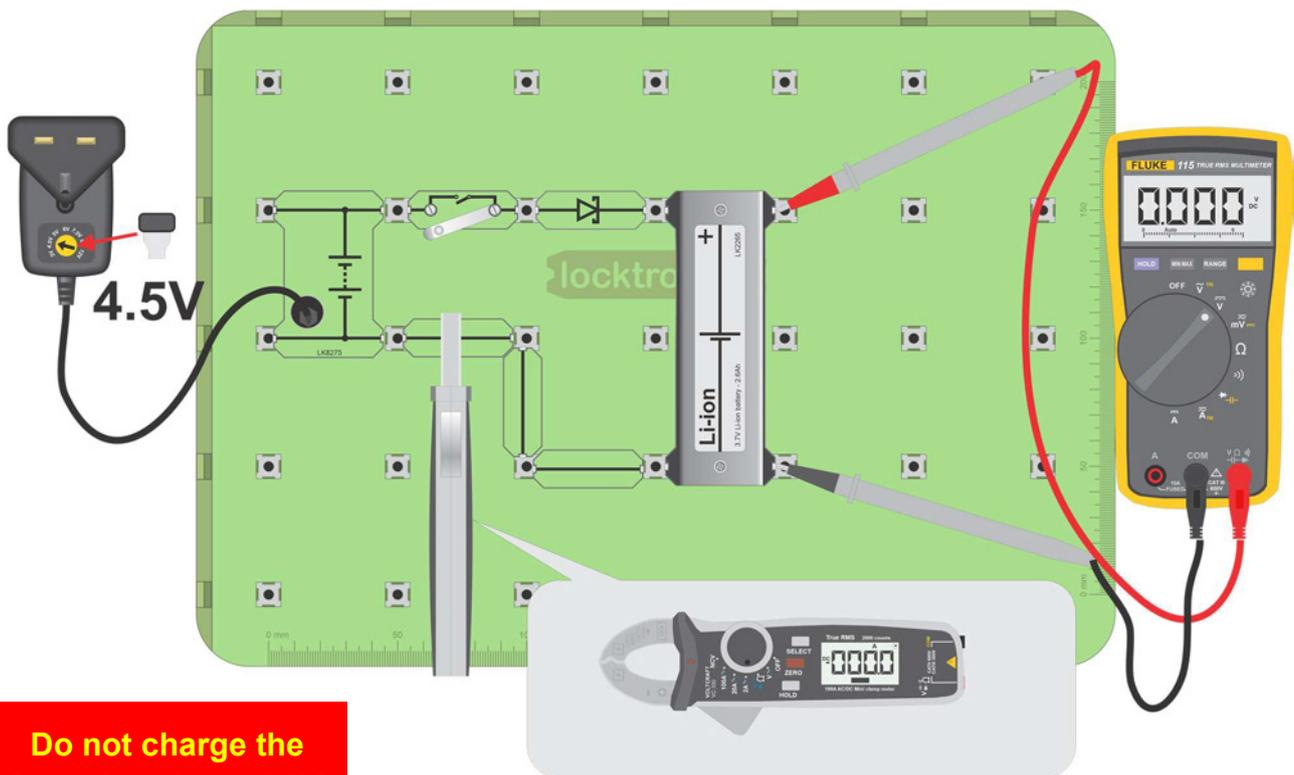
**Do not charge the batteries above 4.2V**
