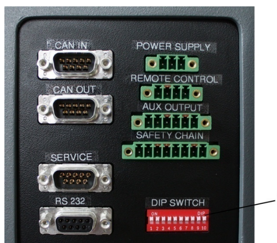
Fig. 10-2 DIP switches on connection panel
